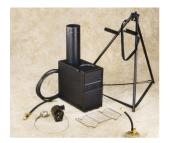
Description: The SHA is a lightweight, portable, multi- fueled (DF-2, DF-1, DF-A, JP-5, JP-8, wood and coal) non-powered heater that provides a maximum heat output of 26,000 BTU with a high/low adjustment capability. The SHA accessories are comprised of the stack, flue cap, gravity feed adapter, fuel can stand and hoses. All accessory components, including the pre-assembled, telescoping stove pipe, can be stored within the heater making it highly mobile and easy to assemble.
